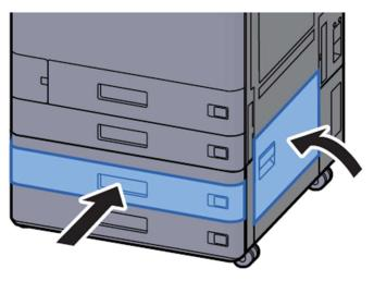
7 If the optional side feeder is installed, return the side feeder to the original position.
