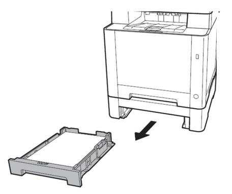
If the machine indicates a jam in section A, remove the paper cassette
