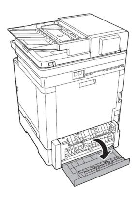
Open the rear Cover Remove any visible jammed paper and close rear cover
