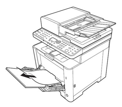
Remove any visible jammed paper from multipurpose tray Remove all paper from multipurpose tray
